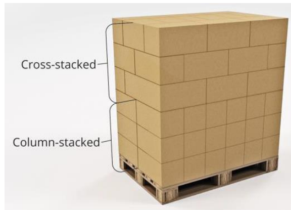
Scheme 1: Explicative scheme of principle of the 3 bottom layers as column stacking
