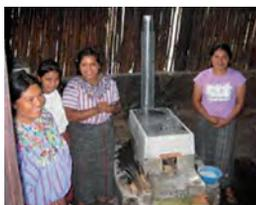
Used in Guatemala, the ONIL stove consists of a fire-clay box which rests inside an insulated stove with a steel chimney. It uses up to 70 percent less firewood than traditional stoves. It has been calculated that women using this stove collect firewood two days less per week. The stove costs US\$87.
