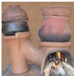
This stove was designed to satisfy the cooking needs of a family of six and to suit the culinary practices and tastes of Sri Lankan people. It burns firewood but also biomass residues such as coconut shells and palm leaves. Fuel efficiency tests have shown that it uses up to 30 percent less firewood than traditional stoves. If correctly insulated with a clay/mud cover, the Anagi stove can be used continuously for three years. Retail price can vary between US\$0.81 and US\$1.80.
