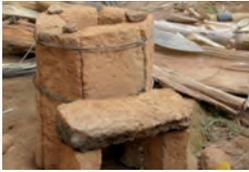
Very easy to build, it requires just five-and-a-half bricks. The half brick is used to construct the opening to the fuel chamber. It uses up to 50 percent less firewood than traditional stoves. It is light and portable, and very cheap. Its price can vary between US\$2 and US\$3.
