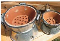
The JIKO stove is used in several African countries, but is most commonly found in Kenya. It is small and portable, reinforced by a metal cladding, and uses between 30 and 40 percent less fuel than traditional stoves. Its cost ranges between US\$4 and US\$6.50.
