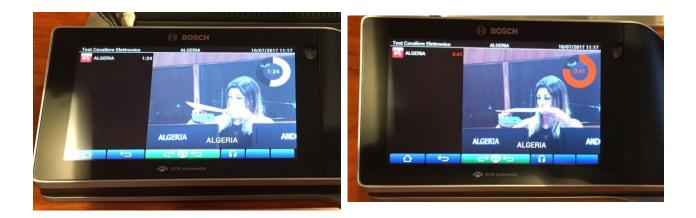
The video microphone system, which was first piloted in January 2017, thanks again to the support of the Government of Italy toward the Landmark HQ renovation project, has a touch screen that allows a delegate to select language and volume, view speakers and speak comfortably from the seat without leaning in due to the wide-range microphone. The photo below highlights features including a clock in the upper right corner to help keep time:
