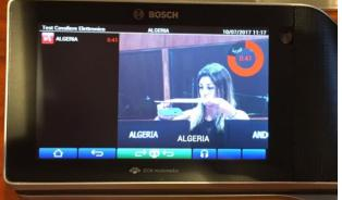
The video microphone system, which was first piloted in January 2017, thanks again to the support of the Government of Italy towards the Landmark HQ renovation project, has a touch screen that allows a delegate to select language and volume, view speakers and speak comfortably from the seat without shifting position due to the wide-range microphone. The photograph below highlights features including a clock in the upper right corner to help keep track of the time:
