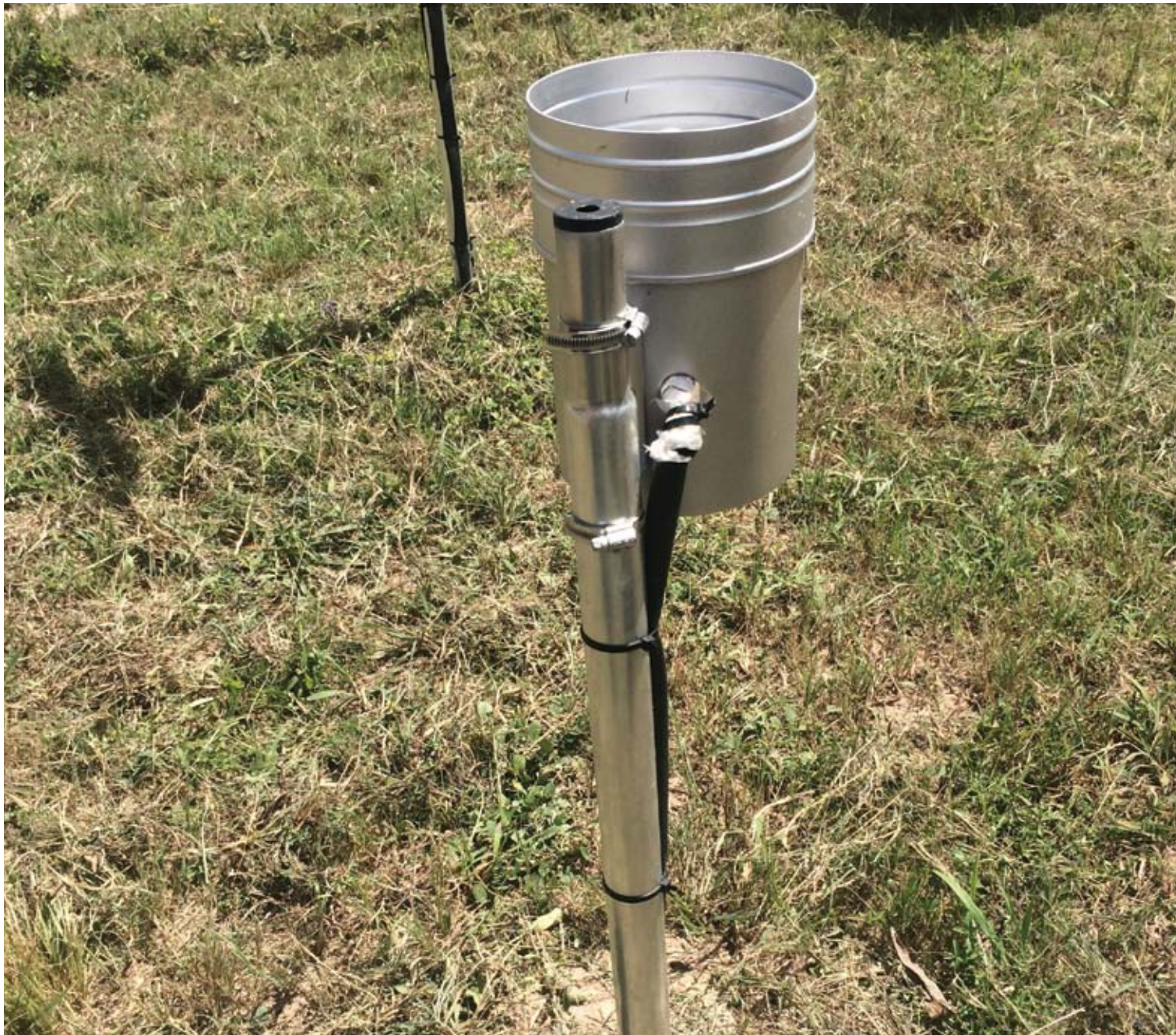
An auto rain gauge at Cheelo weather station in Muzoka, Zambia. WFP/Crissy Mupuchi
