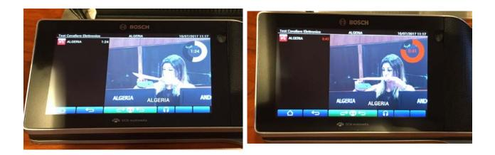
The video microphone system, which was first piloted in January 2017, thanks again to the support of the Government of Italy towards the Landmark HQ renovation project, has a touch screen that allows a delegate to select language and volume, view speakers and speak comfortably from the seat without shifting position due to the wide-range microphone. The photograph below highlights features including a clock in the upper right corner to help keep track of the time:
