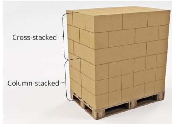
Scheme 1: Explicative scheme of principle of the 3 bottom layers as column stacking
