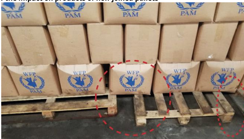
Figure 20. Example of the impact on products of non-joined pallets
