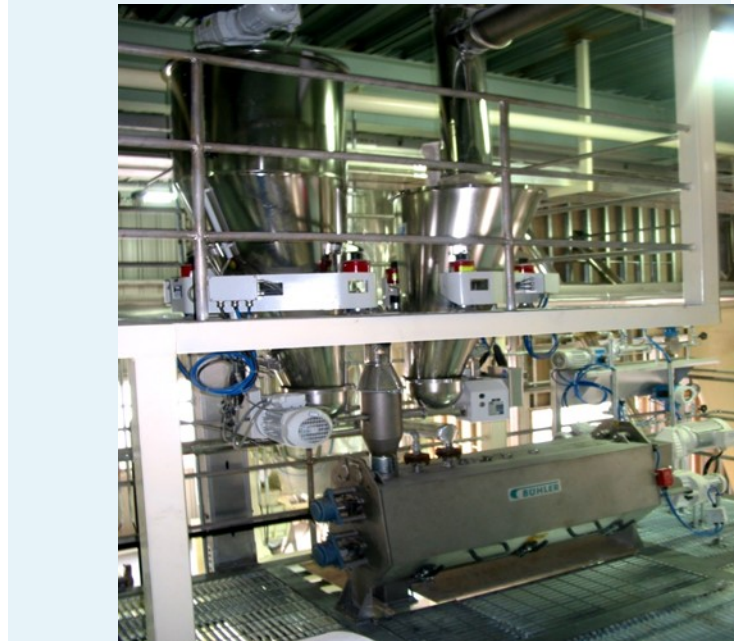
Figure 12: Left - Twin screw extruder for FK - Wenger Mfg Inc. - TX85 - up to 500 kg/h FK, Right - a dosing system for two powder components
