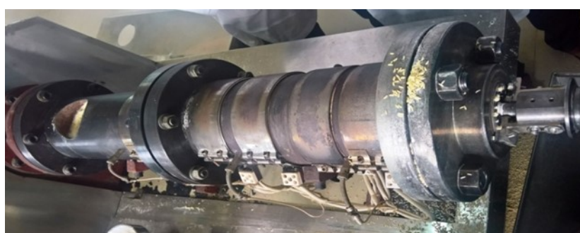
Figure 31: Extruder barrels with external heating shells
