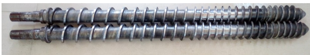
Figure 28: Screw for the warm extrusion process, single piece design without options for changes
