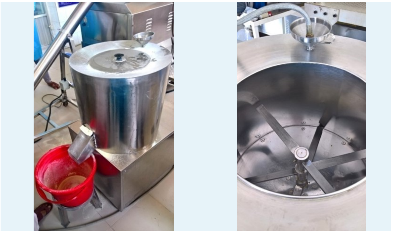
Figure 8: Vertical mixer with a volume for ~25kg batches
