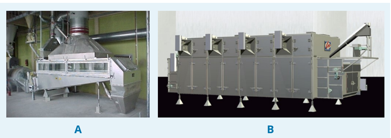
Figure 36: A) Fluid bed dryer "OTW", Bühler AG; B) Belt dryer/cooler "Airflow", Wenger Inc.
