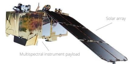
Schematic view of Sentinel-2 satellite spacecraft, deployed by the European Space Agency (ESA)
