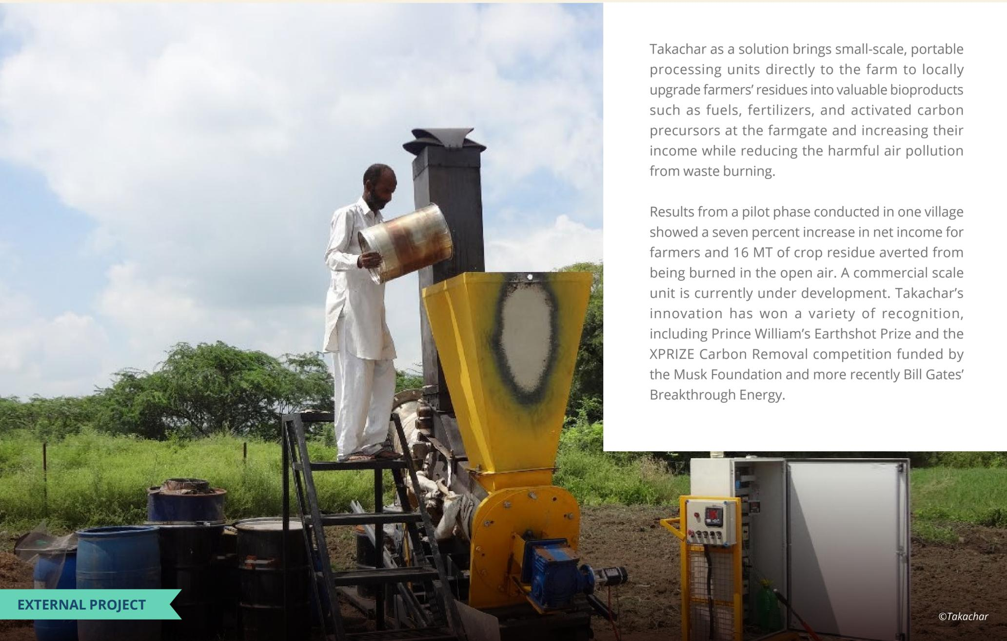
Takachar as a solution brings small-scale, portable processing units directly to the farm to locally upgrade farmers' residues into valuable bioproducts such as fuels, fertilizers, and activated carbon precursors at the farmgate and increasing their income while reducing the harmful air pollution from waste burning.
