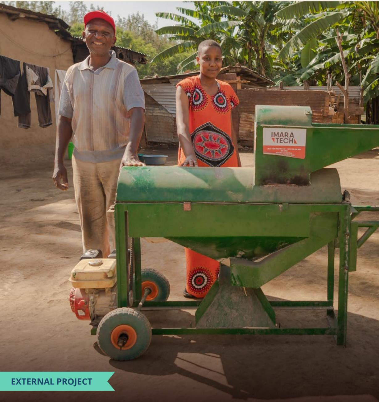
Imara Tech is a Tanzanian start-up that mechanizes small farms with locally made agricultural machines. Imara Tech's first product is a Multi-Crop Threshing (MCT) machine, which threshes staple crops up to 75 times faster than traditional methods. The MCT can be used as an income-generating business, earning operators \$10/hour and saving farmers time and labor.
