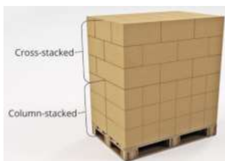
Explicative scheme of principle of the 3 bottom layers as column stacking
