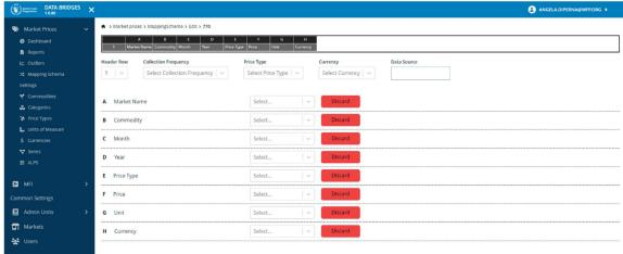
After selecting the header row and specifying the data collection frequency, the app will load the list of columns in the lower part of the screen. Dropdown menus ("Select a mapping") close to the headers will allow to map each column to a series component.
